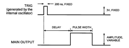
When the ADVANCE/DELAY switch is set to "DELAY", the TRIG output occurs after the main output. This illustrated below:
