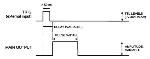
In the "EXT B" mode the instrument is triggered by a TTL-level pulse on the TRIG connector. The output pulse occurs with nominally zero delay, and the output pulse width is approximately equal to the input pulse width. The amplitude is controlled by the front panel settings. This is illustrated below:
