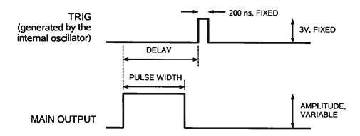
When triggered externally, the TRIG connector acts as an input. In the EXT A mode, the output parameters (pulse width, delay, and amplitude) are determined by the front panel settings. This is illustrated below:
