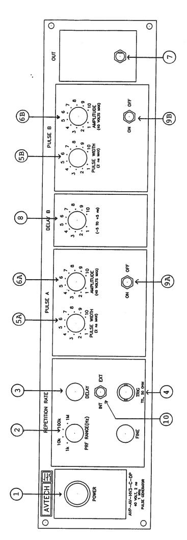
Fig 2: FRONT PANEL CONTROLS
