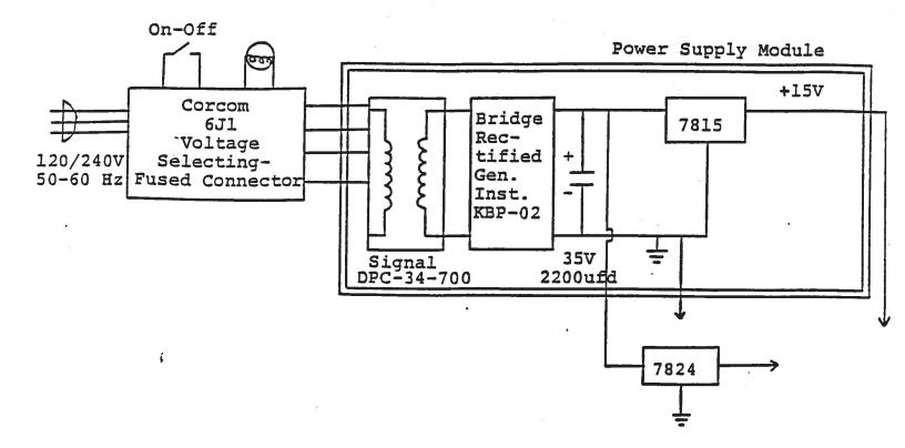
FIG. 5: AVP-2S-PN-EA-EW-EO-C BLOCK DIAGRAM
