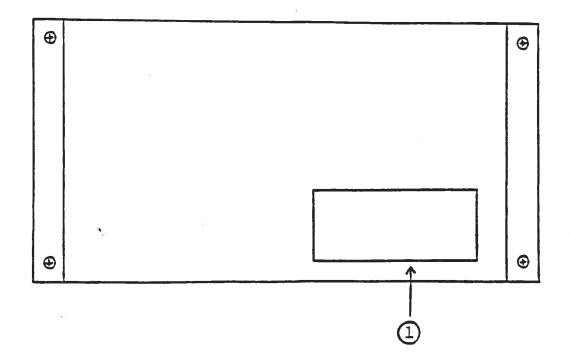
(1) <u>FUSED CONNECTOR, VOLTAGE SELECTOR</u>. The detachable power cord is connected at this point. In addition, the removable cord is adjusted to select the desired input operating voltage. The unit also contains the main power fuse (0.5 A SB). **Fig.** 5
