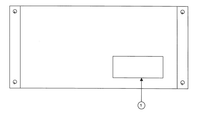
(1) <u>FUSED CONNECTOR, VOLTAGE SELECTOR</u>. The detachable power cord is connected at this point. In addition, the removable cord is adjusted to select the desired input operating voltage. The unit also contains the main power fuse (0.25 A SB).
