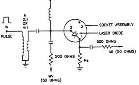
Fig. 3 - AVX-S3 functional equivalent circuit
