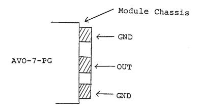
The load should be connected between the OUT and GND terminals using very short leads (<0.5 cm). The voltage across the load may be monitored by connecting a length of 80 mil semi-rigid 50 ohm cable as shown below (or by means of a high impedance scope probe):
