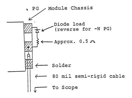
Take care to insure that during soldering the OUT conductor is not shorted to the chassis. Also, use minimal heat when soldering.
