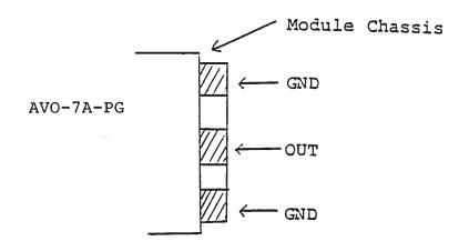
The load should be connected between the OUT and GND terminals using very short leads (<0.5 cm). The voltage across the load may be monitored by connecting a length of 80 mil semi-rigid 50 ohm cable as shown below (or by means of a high impedance scope probe):
