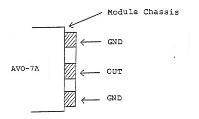
The load should be connected between the OUT and GND terminals using very short leads ( $\leq 0.5$  cm). Take care to insure that during soldering the OUT conductor is not shorted to the chassis. Also, use minimal heat when soldering.
