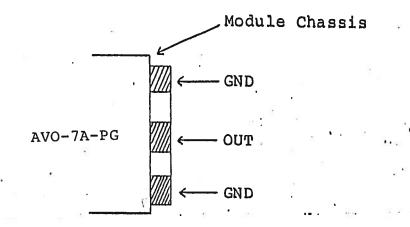
The load should be connected between the OUT and GND terminals using very short leads ( $\leq 0.5$  cm). The voltage across the load may be monitored by means of a high impedance scope probe. The current may be monitored using a current probe or a current transformer arrangement.
