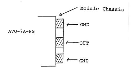
The load should be connected between the OUT and GND terminals using very short leads ( $\leq 0.5$  cm). The voltage across the load may be monitored by connecting a length of 80 mil semi-rigid 50 ohm cable as shown below (or by means of a high impedance scope probe):
