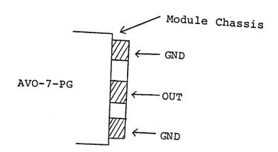
The load should be connected between the OUT and GND terminals using very short leads ( $\leq 2.0 \text{ cm}$ ). The voltage across the load may be monitored by connecting a length of 80 mil semi-rigid 50 ohm cable as shown below (or by means of a high impedance scope probe):
