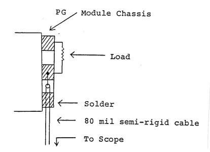
Take care to insure that during soldering the OUT conductor is not shorted to the chassis. Also, use minimal heat when soldering.
