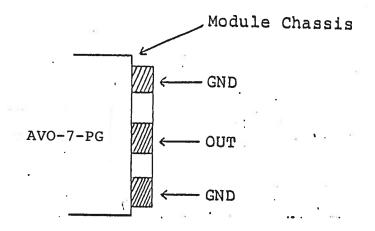
The load should be connected between the OUT and GND terminals using very short leads ( $\leqslant$  0.5 cm). The voltage across the load may be monitored by means of a high impedance scope probe. The current may be monitored using a current probe or a current transformer arrangement.
