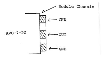
The load should be connected between the OUT and GND terminals using very short leads ( $\leq 2.0 \text{ cm}$ ). The voltage across the load may be monitored by connecting a length of 80 mil semi-rigid 50 ohm cable as shown below (or by means of a high impedance scope probe):
