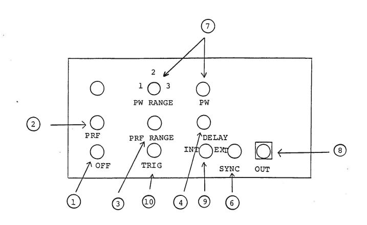
(1) <u>ON-OFF Switch</u>. Applies basic prime power to all stages.
