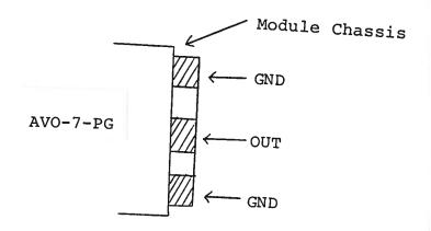
The load should be connected between the OUT and GND terminals using very short leads ( $\leq 0.5$  cm). The voltage across the load may be monitored by connecting a length of 80 mil semi-rigid 50 ohm cable as shown below (or by means of a high impedance scope probe):
