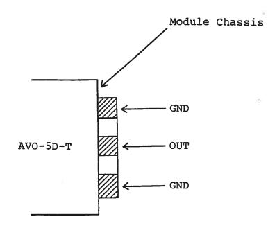
The diode load and series resistor (2.5 to 3.5 Ohm 1/2 W carbon composition resistor) should be connected between the OUT and GND terminals using very short leads ( $\leq 0.5$  cm). The voltage across the resistor-diode load may be monitored by connecting a length of 80 mil semi-rigid 50 Ohm cable as shown below:
