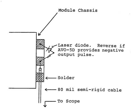
Take care to insure that during soldering the OUT conductor is not shorted to the chassis. Also, use minimal heat when soldering.
