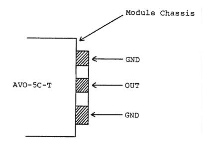
The diode load and series resistor (1.0 to 2.0 ohm 1/4 W carbon composition resistor) should be connected between the OUT and GND terminals using very short leads ( $\leqslant$  0.2 cm). The voltage across the resistor-diode load may be monitored by connecting a length of 80 mil semi-rigid 50 ohm cable as shown below:
