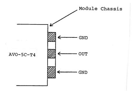
The diode load and series resistor (1.2 to 1.7 ohm 1/4 W carbon composition resistor) should be connected between the OUT and GND terminals using very short leads (< 0.2 cm). The voltage across the resistor-diode load may be monitored by connecting a length of 80 mil semi-rigid 50 ohm cable as shown below:
