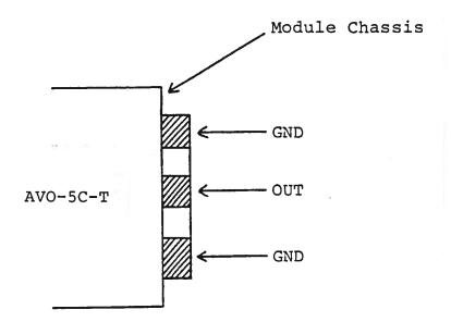
The diode load and series resistor (3 ohm 1/2 W carbon composition resistor) should be connected between the OUT and GND terminals using very short leads ( $\leq$  0.2 cm). The voltage across the resistor-diode load may be monitored by connecting a length of 80 mil semi-rigid 50 ohm cable as shown below:
