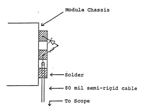
Take care to insure that during soldering the OUT conductor is not shorted to the chassis. Also, use minimal heat when soldering.
