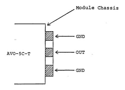
The diode load and series resistor (6 Ohm or 1.5 Ohm 1/2 W carbon composition resistor) should be connected between the OUT and GND terminals using very short leads (≤ 0.2 cm). The voltage across the resistor-diode load may be monitored by connecting a length of 80 mil semi-rigid 50 Ohm cable as shown below:
