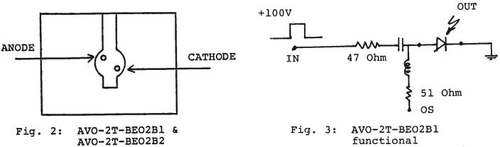
AVO-2T-BEO2B2 output modules PIN socket equivalent circuit
