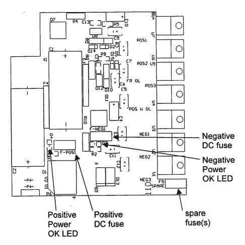
The positive fuse and one of the spare fuses on this circuit board are 1.5A slow-blow fuses, Littlefuse part number R45201.5. (This fuse can be ordered from Digikey, www.digikey.com. The Digikey part number is F1344CT-ND). The negative fuse is a 0.5A slow-blow fuse (Littlefuse R452.500, Digikey part number F1341CT-ND).
