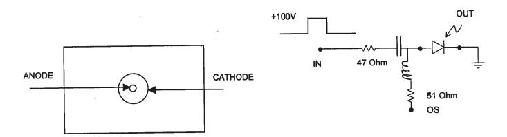
FIG. 1B: AVO-2T-BEO2B3 Output Module PIN Socket
