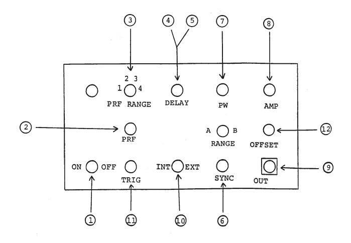
(1) ON-OFF Switch. Applies basic prime power to all stages.
