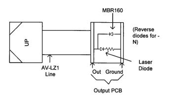
The AV-LZ1 cable inserts into the female out connector on the front panel. It is critically important that the "up" side of the line be visible.
