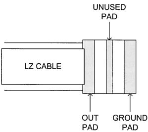
The length of leads used to connect the load to the circuit board should be kept extremely short ( < 0.5 cm), as discussed below.
