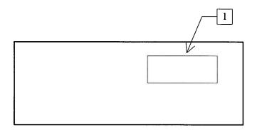
19. <u>AC POWER INPUT</u>. A three-pronged recessed male connector is provided on the back panel for AC power connection to the instrument. Also contained in this assembly is a slow blow fuse and a removable card that can be removed and repositioned to switch between 120V AC in and 240V AC in.
