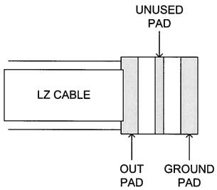
The length of leads used to connect the load to the circuit board should be kept extremely short ( < 0.5 cm), as discussed below.
