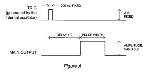
When triggered externally, the TRIG connector acts as an input. The delay controls do not function in this mode.
