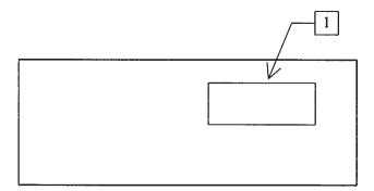
AC POWER INPUT. A three-pronged recessed male connector is provided on the back panel for AC power connection to the instrument. Also contained in this assembly is a slow-blow fuse and a removable card that can be removed and repositioned to switch between 120V AC in and 240V AC in.
