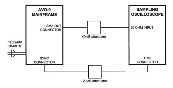
Since most sampling oscilloscopes have limited input amplitude ranges, attenuators are required.
