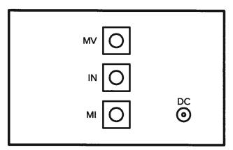
**AVX-S1 OUTPUT MODULE, CONNECTOR VIEW**
