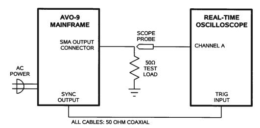
Since the AVO-9A-C-P-P2-LARB can generate pulses with rise times as low as 200 ps, it may be necessary to use a sampling oscilloscope, rather than a real-time
