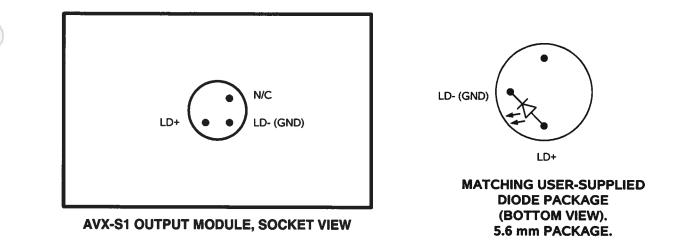
**NOTE:** Trim the diode leads to **no longer than 1.0 cm in length**. If the leads are longer than that, they may cause an internal short circuit in the output module, which may cause damage to the diode and the output module.
