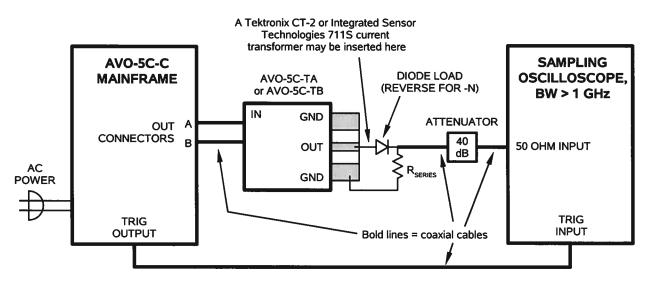
The attenuator is required to prevent damage to the sampling oscilloscope.
