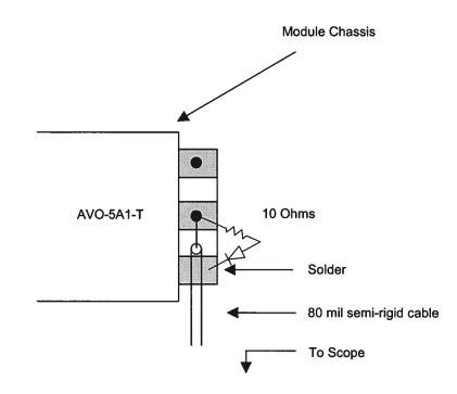
Take care to insure that during soldering the OUT conductor is not shorted to the chassis. Also, use minimal heat when soldering. The series resistor may be varied between about 7 to 15 Ohms with minimal waveform degradation.
