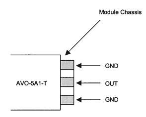
The diode load and series resistor (10 Ohm 1/4 W carbon composition resistor) should be connected between the OUT and GND terminals using very short leads (< 0.2 cm). The voltage across the resistor-diode load may be monitored by connecting a length of 80 mil semi-rigid 50 Ohm cable as shown below:
