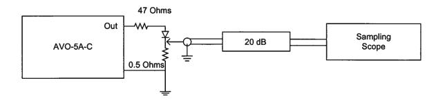
The output current may be observed by placing a 0.5 Ohm carbon composition resistor in series with the diode and placing a 50 Ohm cable across this resistor.
