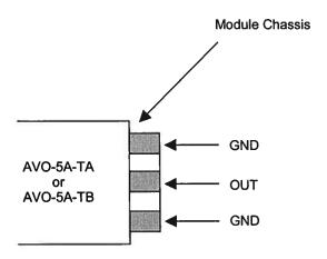
The diode load and series current limiting resistor should be connected between the OUT and GND terminals using very short leads (<0.5 cm). The series current limiting resistors must be non inductive. Carbon composition resistors are suitable for this application. The voltage across the resistor-diode load may be monitored by means of a high impedance scope probe.
