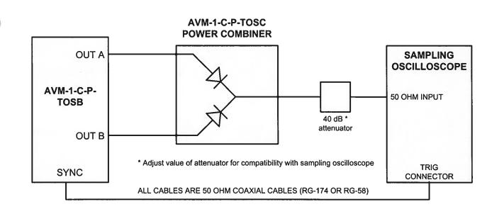
In this mode, the AVM-1-C-P-TOSC combines the OUT A and OUT B signals into a composite output, as shown below.
