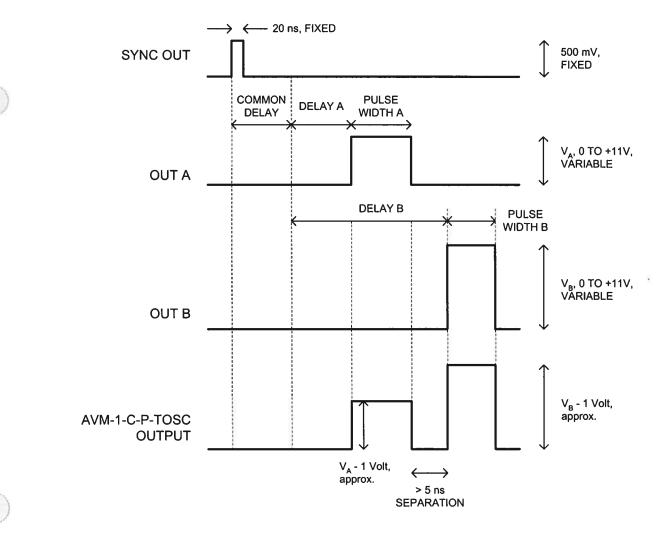
For proper operation, the two delay controls of the AVM-1-C-P-TOSB must be set such that the leading edge of the second pulse is 5-20 ns after the falling edge of the first pulse.
