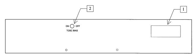
1. <u>AC POWER INPUT</u>. A three-pronged recessed male connector is provided on the back panel for AC power connection to the instrument. Also contained in this assembly is a slow blow fuse and a removable card that can be removed and repositioned to switch between 120V AC in and 240V AC in.
