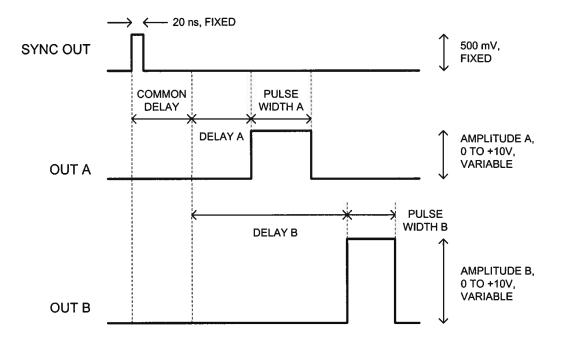
The pulse width, amplitude, and delay of each channel are independently variable. A variable common delay is also present. When triggered externally, the operation is similar, except that no SYNC pulse is generated.
