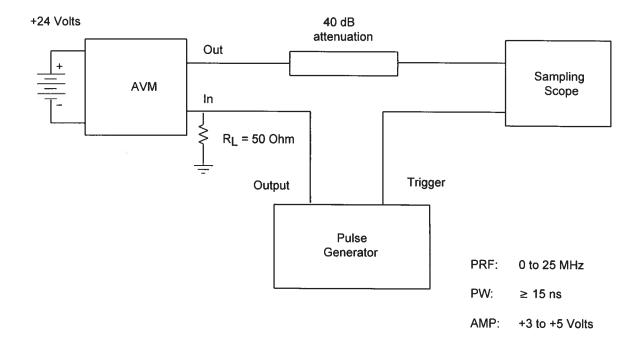
Power line: +24 Volts/0.50 Amps DC, shielded twisted pair, < 3 meters
