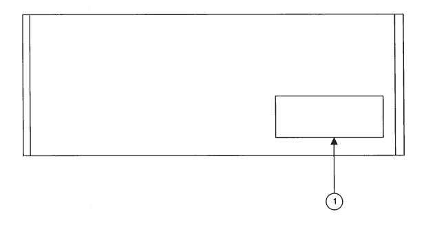
(1) <u>FUSED CONNECTOR, VOLTAGE SELECTOR</u>. The detachable power cord is connected at this point. In addition, the removable cord is adjusted to select the desired input operating voltage. The unit also contains the main power fuse (0.5 Amp).
