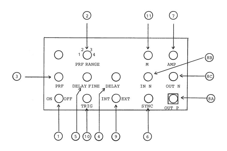
(1) <u>ON-OFF Switch</u>. Applies basic prime power to all stages.
