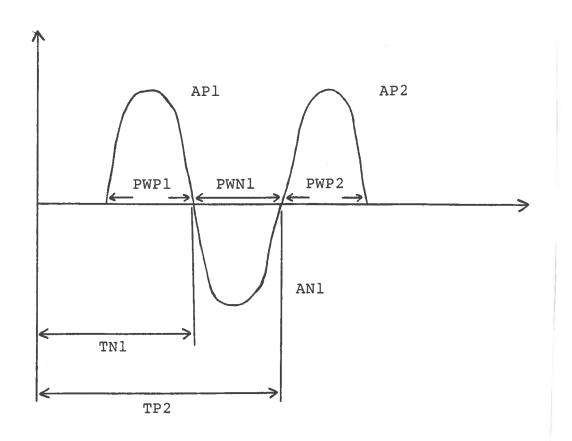
Fig. 3 OUTPUT WAVEFORM FORMAT AND VARIABLE PARAMETERS
