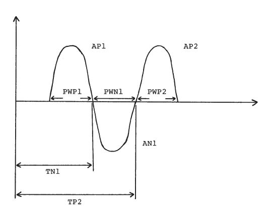
Fig. 3 OUTPUT WAVEFORM FORMAT AND VARIABLE PARAMETERS
