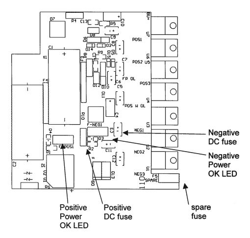
The positive fuse and the spare fuse on this circuit board are 1A slow-blow fuses, Littlefuse part number R452001. (This fuse can be ordered from Digikey, www.digikey.com. The Digikey part number is F1343CT-ND). The negative fuse is a
