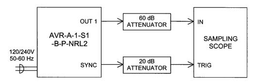
BASIC TEST ARRANGEMENT FOR TESTING CHANNEL 1
