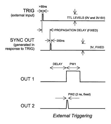
As before, if the delay is negative, the order of the SYNC and OUT pulses is reversed.
