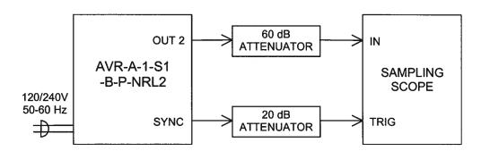
BASIC TEST ARRANGEMENT FOR TESTING CHANNEL 2
