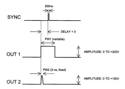
Basic Output Pulses for Delay < 0
