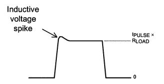
Attaching a current transformer (for measuring current waveforms) can add significant inductance, because of the necessary wire length that must be fed through the transformer. (The Pearson 2878 requires approximately 1.5".) For this reason it is recommended that the optional self-contained current transformer ("M") be used.
