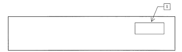
1. AC POWER INPUT. A three-pronged recessed male connector is provided on the back panel for AC power connection to the instrument. Also contained in this assembly is a slow-blow fuse and a removable card that can be removed and repositioned to switch between 120V AC in and 240V AC in.
