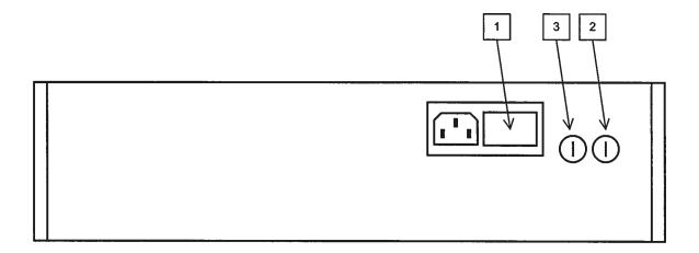
AC POWER INPUT. A three-pronged recessed male connector is provided on the back panel for AC power connection to the instrument. Also contained in this assembly is a slow-blow fuse and a removable power selector card that can be removed and repositioned to switch between 110-120V AC in and 220-240V.
