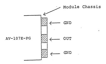
The load should be connected between the OUT and GND terminals using very short leads ( $\leqslant$  2.0 cm). The voltage across the load may be monitored by connecting a length of 80 mil semi-rigid 50 ohm cable as shown below (or by means of a high impedance scope probe). The current may be monitored using a current probe such as the TEKTRONIX Model CT-2.
