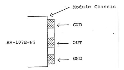
The load should be connected between the OUT and GND terminals using very short leads ( $\leqslant$  2.0 cm). The voltage across the load may be monitored by connecting a length of 80 mil semi-rigid 50 ohm cable as shown below (or by means of a high impedance scope probe). The current may be monitored using a current probe such as the TEKTRONIX Model CT-2.
