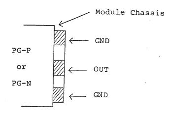
The load should be connected between the OUT and GND terminals using very short leads ( $\langle 0.5 \text{ cm} \rangle$ .
