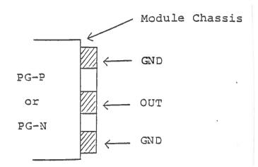
The load should be connected between the OUT and GND terminals using very short leads ( $\leq 0.5$  cm). (See 11).
