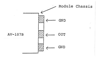
The load should be connected between the OUT and GND terminals using very short leads ( $\leqslant$  0.5 cm). The voltage across the load may be monitored by connecting a length of 80 mil semi-rigid 50 ohm cable as shown below (or by means of a high impedance scope probe). The current may be monitored using a current probe such as the TEKTRONIX Model CT-2.
