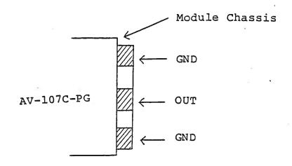
The load should be connected between the OUT and GND terminals using very short leads ( $\leq 0.5$  cm). The voltage across the load may be monitored by connecting a length of 80 mil semi-rigid 50 ohm cable as shown below (or by means of a high impedance scope probe). The current may be monitored using a current probe such as the TEKTRONIX Model CT-2.
